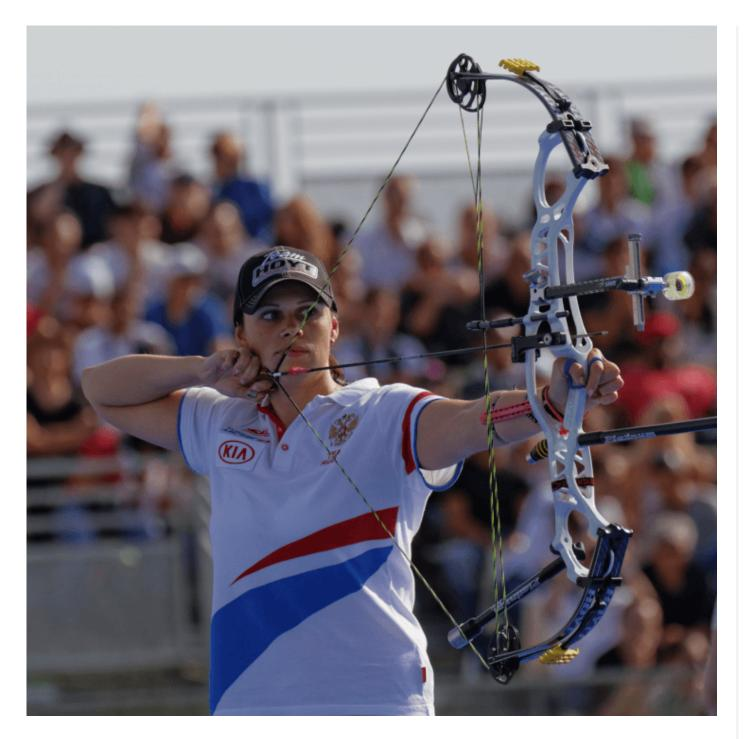
If you look at the top and bottom of the bow, you'll see that there are rounded wheels that hold the draw string. These are called "cams." They are part of a levering system that includes cables and pulleys that allows the bow to multiply (or "compound") the force used to push the arrow forward.
