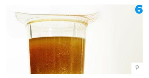
**6.** Allow the fuel to air out for a day or two with the top off to let any cloudiness (caused by a small amount of remaining water) dissipate.
