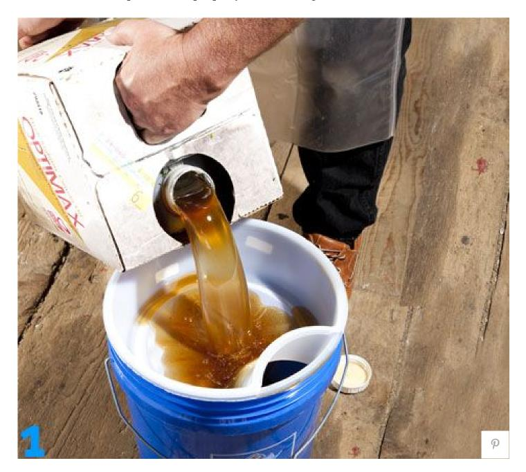
1. Start by filtering your waste vegetable oil to remove chunks of food left over from the fryer. We used a paint filter. The filtrate is mostly breading, with the occasional chunk of ... something. Mix all your oil from different sources to achieve a uniform sample.
