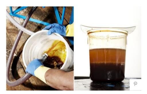
**5.** Drain the glycerin from the bottom until you get lighter-colored, thinner biodiesel pouring from the valve. Then use water to wash the excess methanol, lye and soapy residue from the biodiesel. The water will settle to the bottom of the vessel in a few hours, where you can drain it out.
