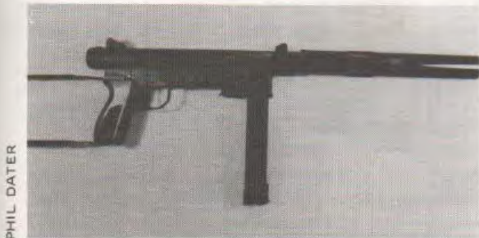
PHIL DATER Phil Dater has standardized his 9mm suppressor as the SG9, adaptable to any 9mm submachine gun. It's shown here on a S & W M76.
