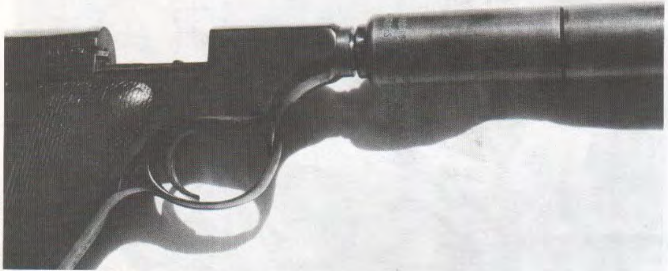
Side view of the .22 caliber Woodsman with the Gold Spot suppressor in place.
