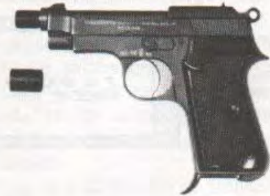
Beretta .22 with extra length bushing and thread. The end cap is a thread hider which can be screwed onto the thread when not using suppressor
