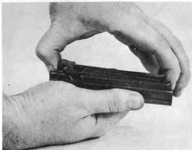
FIGURE 65. REMOVING BOLT FROM SLIDE.
