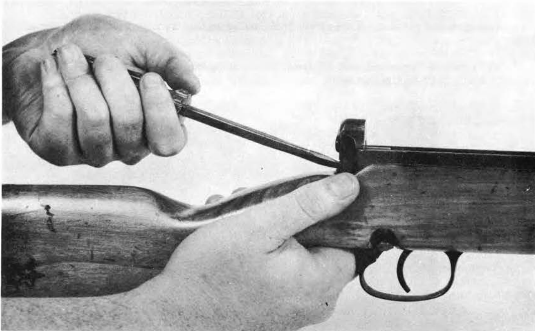
FIGURE 66. REMOVING TRIGGER MECHANISM (STEP 1).
