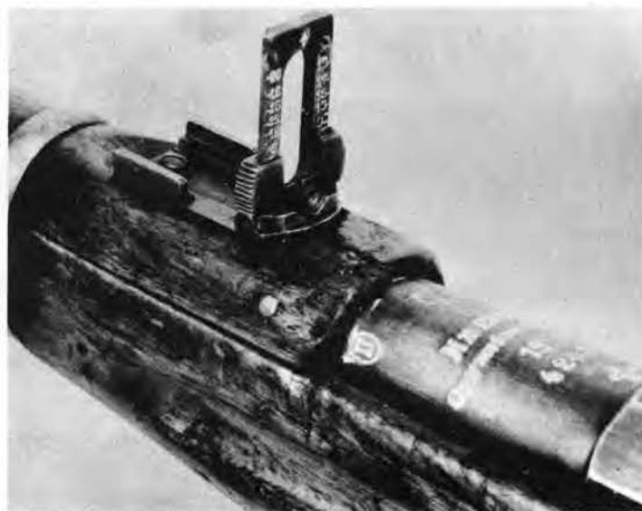
FIGURE 15. REAR SIGHT FOR CARBINE M1910.
