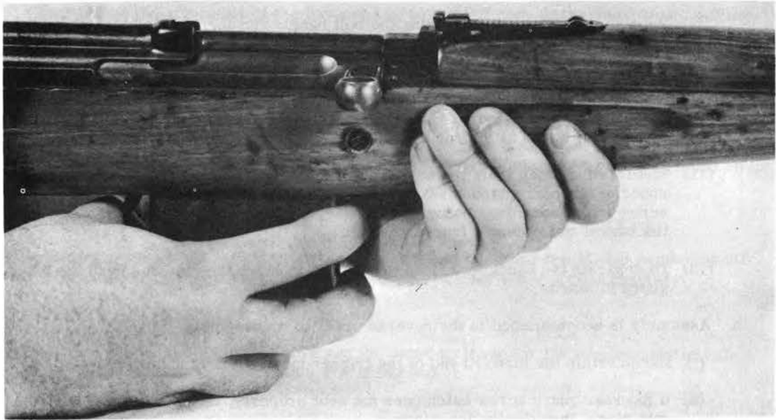
FIGURE 60. REMOVING MAGAZINE FROM TOKAREV RIFLE.
