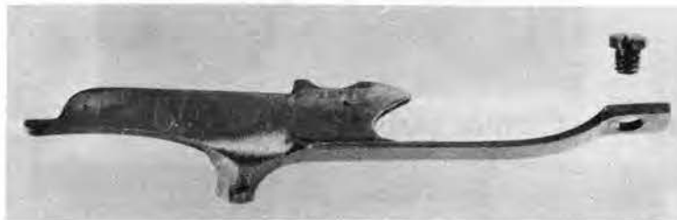
FIGURE 12. INTERRUPTER-EJECTOR FOR RIFLE M1891.
