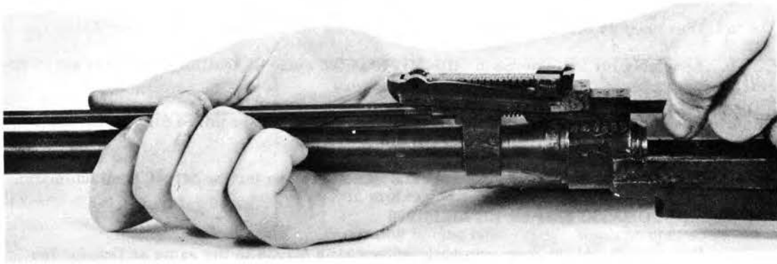
FIGURE 73. REMOVING THE OPERATING ROD
