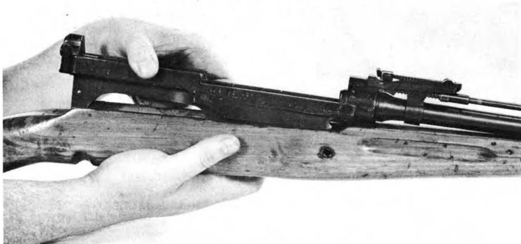
FIGURE 72. LIFTING THE RECEIVER AND BARREL OUT OF THE STOCK.
