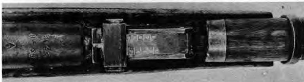
FIGURE 31. REAR RAMP SIGHT FOR CARBINE M1938.
