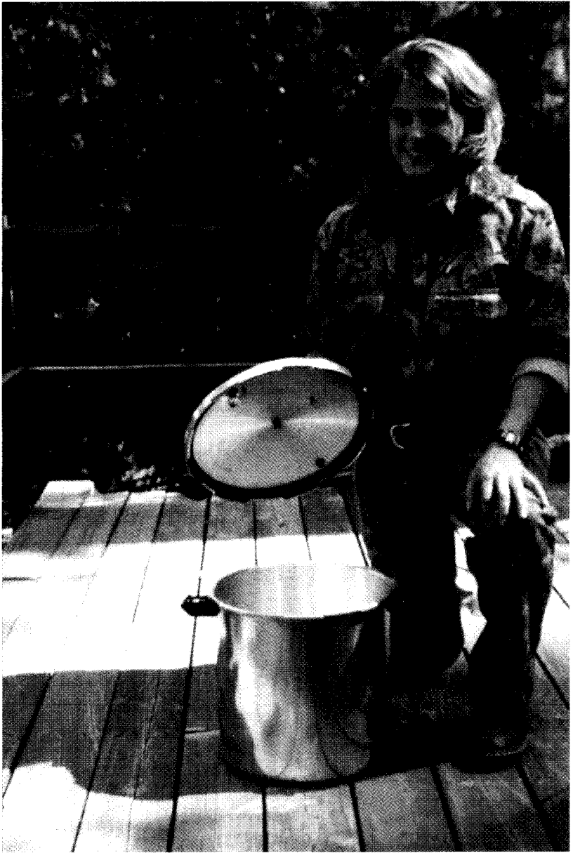
A relatively small 7-quart pressure pot useful for canning as a type of autoclave.
