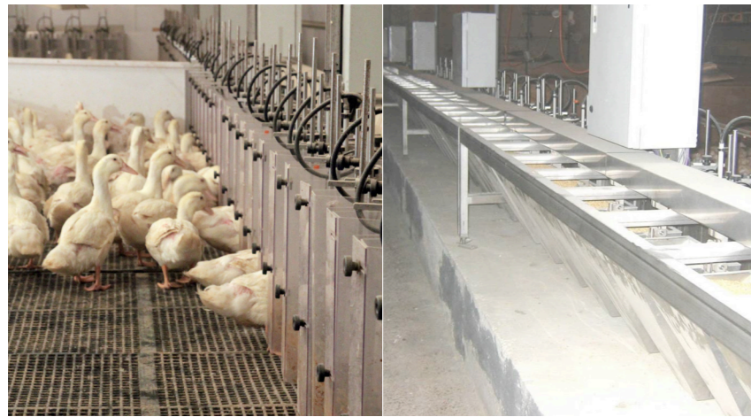
Fig. 4 & 5: Feeding Station to measure individual feed intake in free moving flocks. Left: Entrance of the feeder station is designed so that only one duck has access to the feeder. Ducks in the feeding station are identified using RFID technique. Right: Feed hoppers are fitted to electronic scales. Feed consumption is being recorded and stored on a PC.
