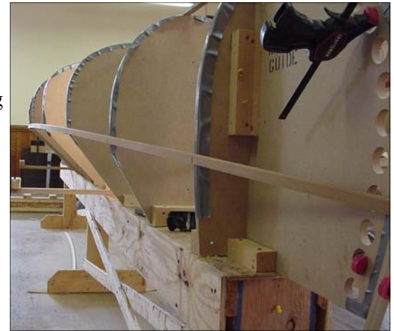
Sight down the sheerline strip from the bow or stern to ensure it's fair.
