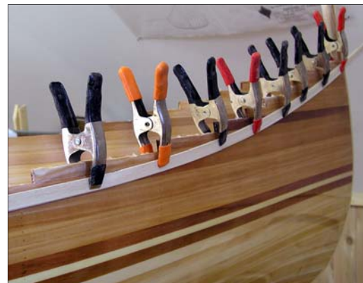
Use an extra strip to mark the sheerline before cutting with a saber or pull saw
