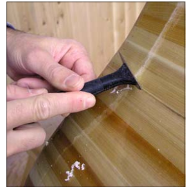
A scraper easily removes lumps and drools in the green stage of curing
