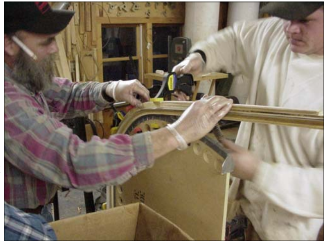
Jim and Jeremiah bending ash stems around the stem forms. They have spread thickened epoxy between laminations and separated the inner and outer stems with a piece of plastic.
