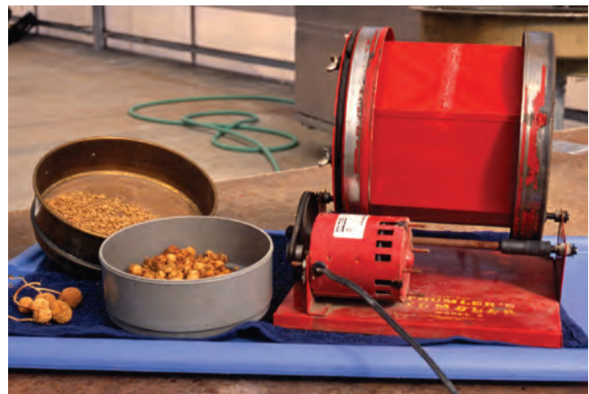
Figure 9.4 —Hobby-size rock tumblers can be used to scarify seeds and avoid seed destruction that can occur with sulfuric acid or heat scarification. Photo by Tara Luna.
