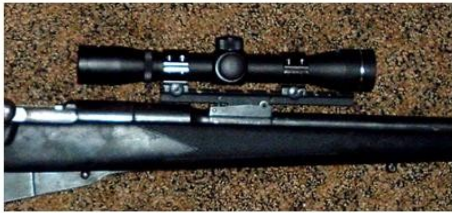
Mosin-Nagant with rear sight scope mount. This will not get in the way of operating the bolt.
