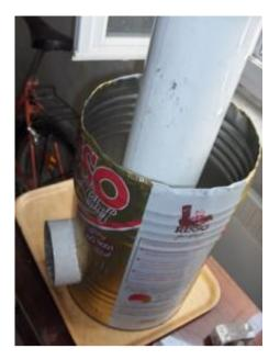
Then I took that same thin strip of wood, drew a little line on it the same length for the stove pipe I'd marked, and then continued drawing the line around the pipe using the length of wood and its marker to keep the line even all the way round. A tape measure could also have been used, but I was too lazy to go and get it out of my tool box....
