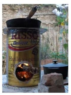
The twigs can be set alight by placing a handful of straw in the pipe's elbow, adding more straw if they are slow to take. With long sticks, bricks can be placed underneath them for support. When you want to put the twigs out, have a little pot with sand handy to plonk them into.
