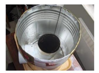
Then I slotted in my straight length of stove pipe onto the elbow. I wanted the central pipe to sit about two or three cm below the rim of the outer tin, so I rested a thin length of wood from the outer edge to the central column, inclined it down the pipe a couple of cm and marked that point with a pen.
