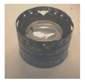
The stand serves several purposes. It reflects heat in, it acts as a wind shield, and it holds the pot. When cool, it can hold the stove for packing. It is handy to have a glove to use a hot mitt (to lift hot pots form the stove), to extinguish the stove (quickly smother the fire and little damage should result to the glove), and also act as a cushion to keep the stove from rattling in the pot stand when packed.
