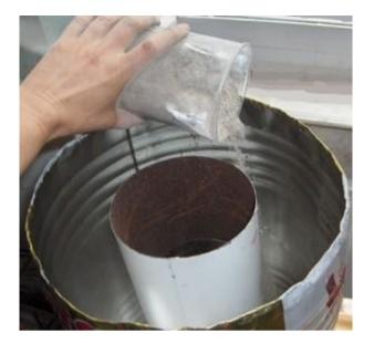
I filled it to a level that left a depth of about 8 or 9cm from the outer tin's top rim to the surface of the ash.
