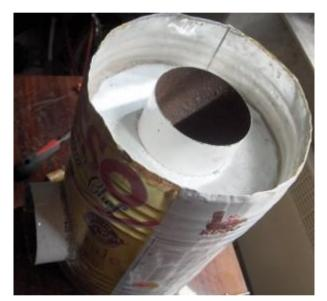
Now the final touches, putting in the stove's twig shelf. You cannot just put the twigs straight into the stove pipe without a shelf because they need to be raised in order to allow air to flow underneath, as with a vent, to get the fire going. I could have used the tin top but I used another scrap of tougher tin I found lying around. This shelf has to be long enough to hold the twigs but not so long that it intrudes into the bent part of the pipe's elbow, that's where the flames belong.
