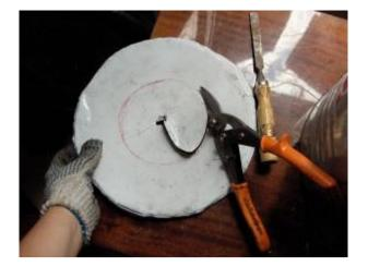
....filed off the rough edges and slotted it into place over the central stove pipe. This keeps the pipe in place and holds the ashes down. I did a rough job (I'm a beginner after all) and there is a little ash around some of the edges still, but this doesn't affect the efficiency of my stove at all.
