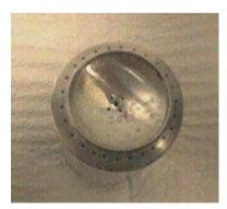
Take the can with the holes and cut off the bottom, about 1 inch up from the bottom. Cut ½ inch slits around the cut edge, about every half inch.
