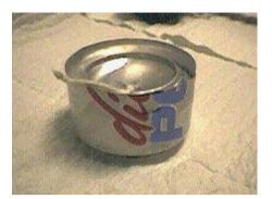
The fuel (alcohol) is poured into the top of the can. This will soak the string, which will act as a wick. The purpose of the wick is to keep the flame going until the alcohol is warm enough to stay lit. The wick is our primary contribution to the coke can design.
