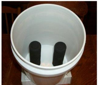
Assemble the filter by placing the upper bucket on the lower. Be sure to line up the holes so the tubes extend through the lid of the lower bucket. Place the remaining lid on top.
