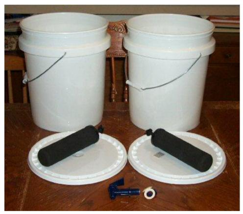
Drill two 1/2" holes in the bottom of the upper bucket and two matching holes in the lid of the lower bucket.
