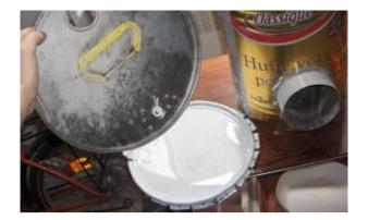
I measured the diameter of the rocket stove's outer tin and cut out a circle from the tin lid with the same diameter. Luckily for me, the interior line of the lid was almost exactly the same diameter so I didn't need to draw a line. Had I not had that stroke of luck, I'd have put the rocket stove onto the lid, traced a line around its base, and cut the circle a few milimetres inside the line to compensate for the difference in diameter between the outside of the tin and the inside.
