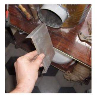
I cut it with folded-down edges so that it could be wedged into the pipe quite firmly.
