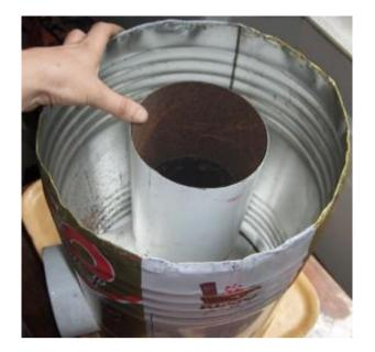
Just in case, I got David to file off with the disk saw the enamel and paint where the pipe comes through the bottom hole because I was in two minds about filling the slightly uneven gaps (I'm no expert with those tin snips!) with some type of soldered metal...but in the end, the ash insulation is tightly packed and doesn't fall out as long as you don't knock the stove around. In this photo below you can see how the final stove pipe looks with elbow and vertical piece slotted together.
